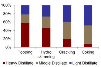
Figure 2.3: Yield from different refinery types
